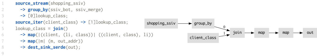
Figure 5: Push Group By Through Join
